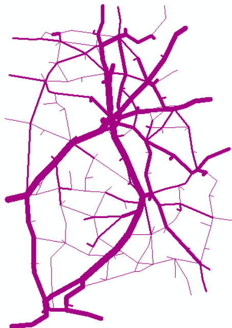
FIGURE 9 Assignment to the Network with Line Thickness Proportional to Assigned Volume.
